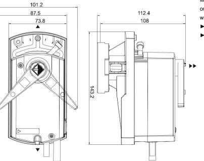
Minimumdistance from walls or ceilings during mounting, wiring, operation, etc. ► = > 100 mm
